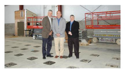
A "strong floor", is a steel, reinforced-concrete slab, which is 82 feet long by 22 feet wide with concrete 3.5 feet deep. Additionally, it has metal anchor plates laid out on a square grid containing 3-foot-long, 50,000-pound-capacity bolts spaced every 3 feet on center along the surface so that test structures could be bolted to the floor.
